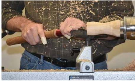
2. Beginning to hollow the body. Make an indent to take a Forstner bit to grub out most of the interior.
