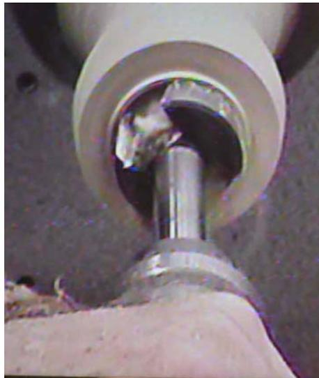
5. Clearing the interior with a Forstner bit—saves a lot of hand-gouging.
