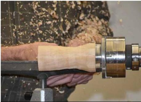
1. Start with a block about 2X the length of the finished body. Start forming it to a long oval with a spindle point.
