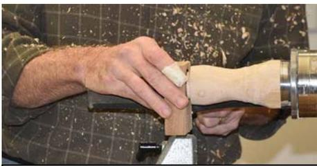
4. Using a gauge drilled with the same Forstner bit as the roof cavity.
