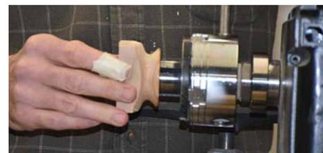
6. The roof is reversed onto a pin jaw chuck.
