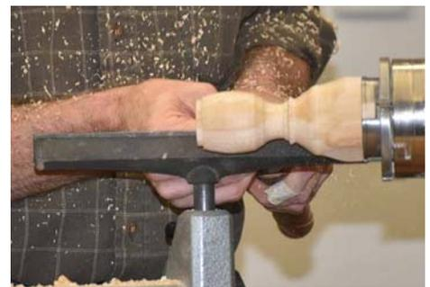
6. Defining the outside of the body. Starting to work toward the finished shape of the spindle bottom.
