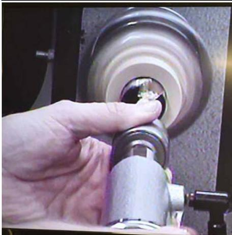
3. The cavity is formed with a Forstner bit.
