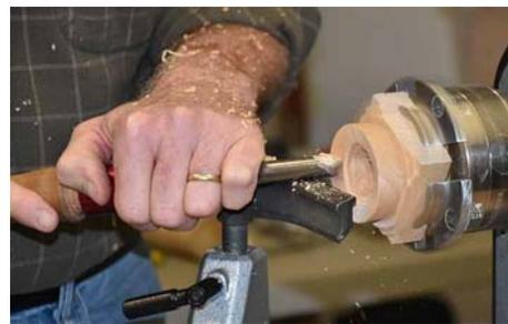
4. Using a gouge to create the underside of the roof and hollow out the roof cavity to make it as light as possible. A ridge is left inside for the body to butt against.
