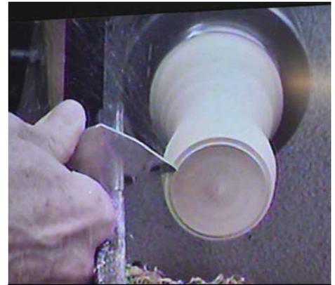
3. Randy uses a parting tool to define a ridge which will pressure-fit the roof cavity.
