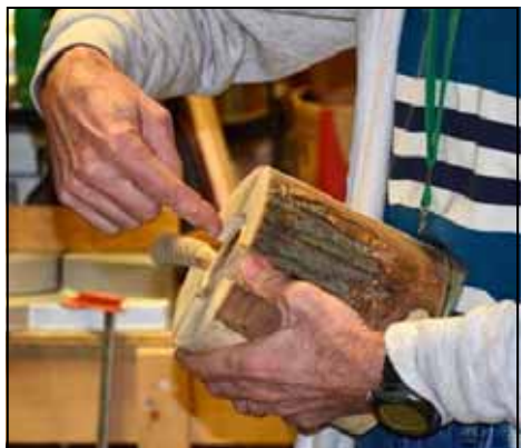
Using a special jam chuck to hollow out a ladle.
