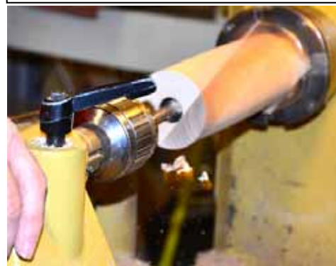
Boring the candle socket in a fancy candlestick.
