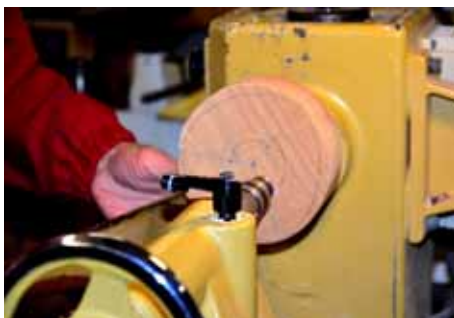
Set up on one of the 3 offset centers.
