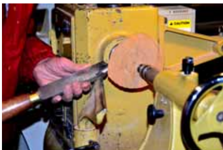
Preparing to scrape the first side smooth. Approach the piece gently. It's nearly impossible to get back to an offset center, so do all steps in sequence on each side.
