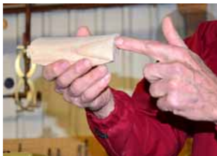
This object was turned using 2 axes between dead and live centers.
