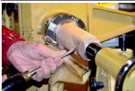
Turning the cup for the candle. The Forstner bit has been exchanged for a cone center.
