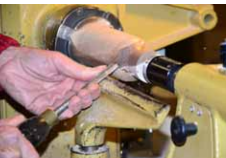
Turning the first segment. Russ uses a spindle gouge with a steep shape.—about 60 degrees.
