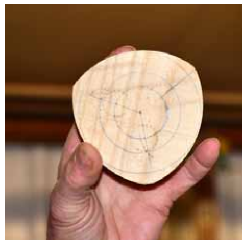
A simple form using 3 parallel axes.
