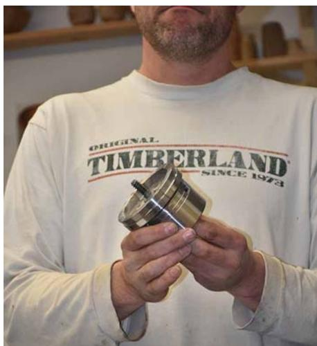
The "screw chuck" is held in a 4-jaw chuck. The work piece is screwed down to make contact with the jaws.
