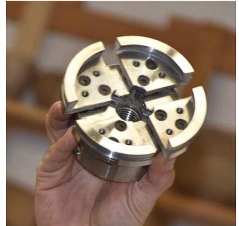
4-jaw chucks can have flat jaws or, like this one, dovetail-jaws. The bowl tenon should be cut to match the type of jaw.
