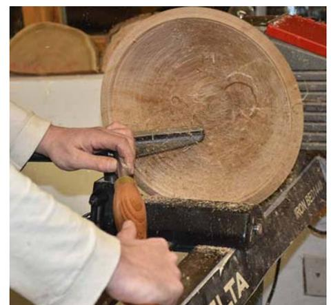
Making the interior cuts: The tool rest is close to the surface and below center enough so the tool is at center when presented to the wood. The tool bevel should ride on the wood and the cutting point back from the point slightly.
