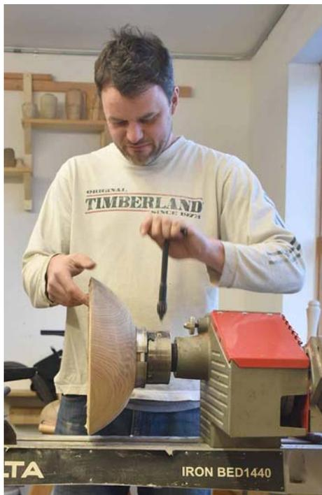
Nick feels the best way to deal with turning errors is to avoid them. He started with proper mounting on the lathe.
