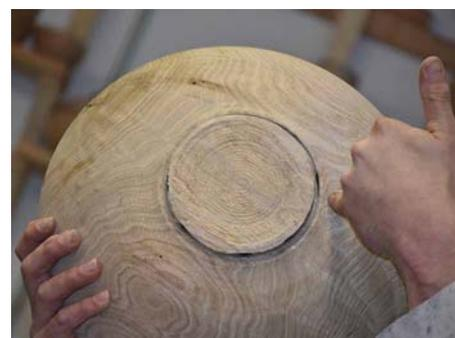
By cutting the tenon to fit the jaws, both inside and top, you get maximum bearing surface, and maximum grip. This resists having the workpiece pull away under heavy cutting.
