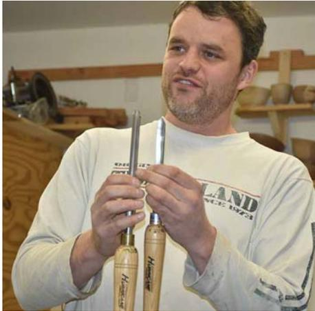
Use the right gouge for the job you want to do. The bowl gouge has a deeper flute than the spindle gouge. Never use a spindle roughing gouge for bowls.
