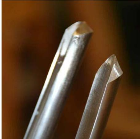
The bowl gouge on the left has a deeper flute than the spindle gouge on the right. Its cutting angle can be from 35 degrees to 75 degrees, depending on the wood you will use it on.
