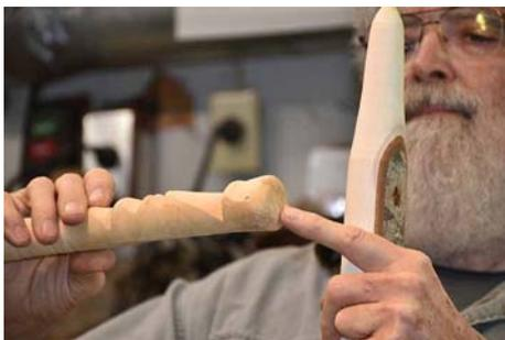
7. Roughly half-way between the real center and the back edge should be the 2nd center, raising the opposite side so you can define the facial features.
