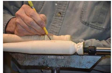
9. Define the top of the stake. Figure and mark the length for the figure's brow, nose, and mouth.
