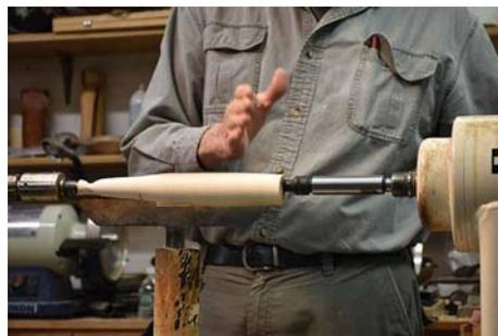
8. Re-mount the workpiece using the 2nd center.
