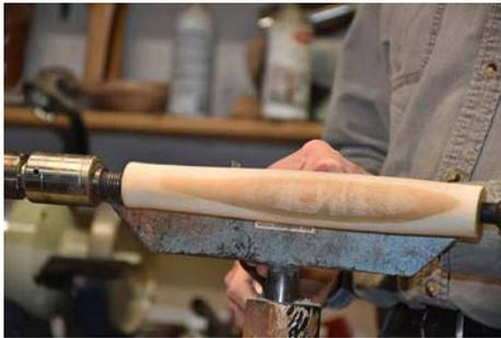
4. Start turning so the workpiece is partially round.
