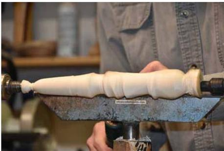
16. The last steps are to get the point final tapered, and to round off the top, removing both mounting points. Sanding will help keep splinters down when the stake is out in the weather.
