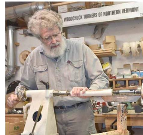
3. Mount the workpiece between centers on the lathe. Dick uses a cup center on each end and adds enough pressure so the tool can cut.
