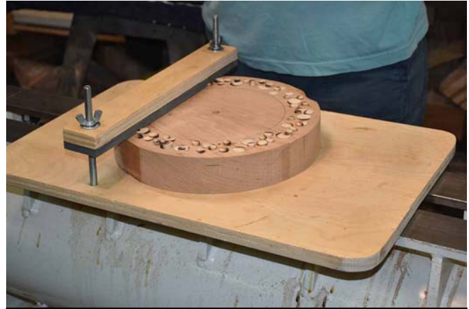
This hold-down fixture can be used with a drill press or router to provide precise positioning without marring surfaces. Items used: 3/8" threaded rod, nuts & wingnuts, rigid foam and 3/4" plywood or thicker.
