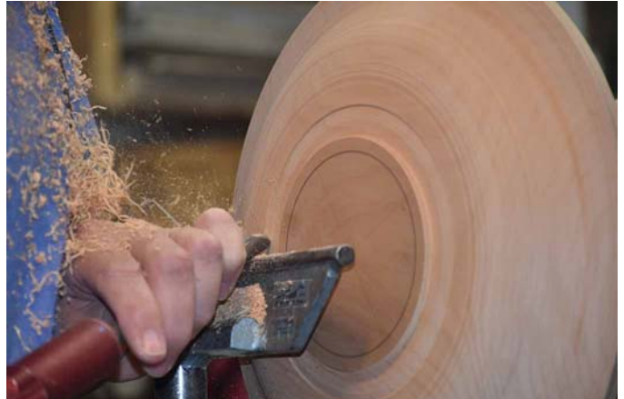
Forming the outside of the platter. Careful work here with a sharp tool avoids tearout and gives a tenon to grip for turning the face side.
