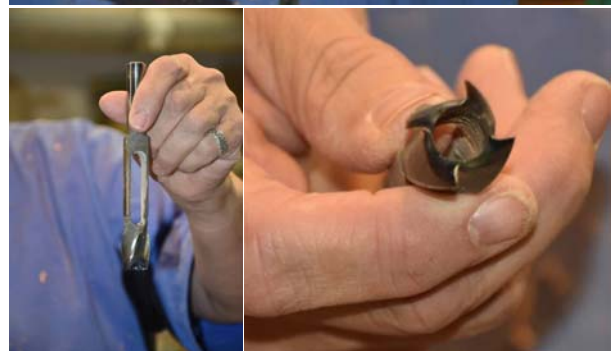
To make the shaded inserts, Janet uses a plug cutter in light colored wood. The plugs are partially buried in very hot sand and allowed to toast for varied periods. For more detail, see the attached PDF from the AAW magazine.
