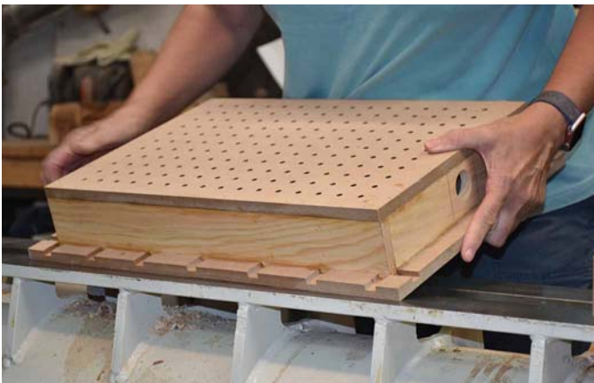
(left) The vacuum platform is formed, top & bottom, from MDF. Janet has access to CNC machines to drill the hole array. It is internally braced. The shopvac is cheap & powerful enough.
