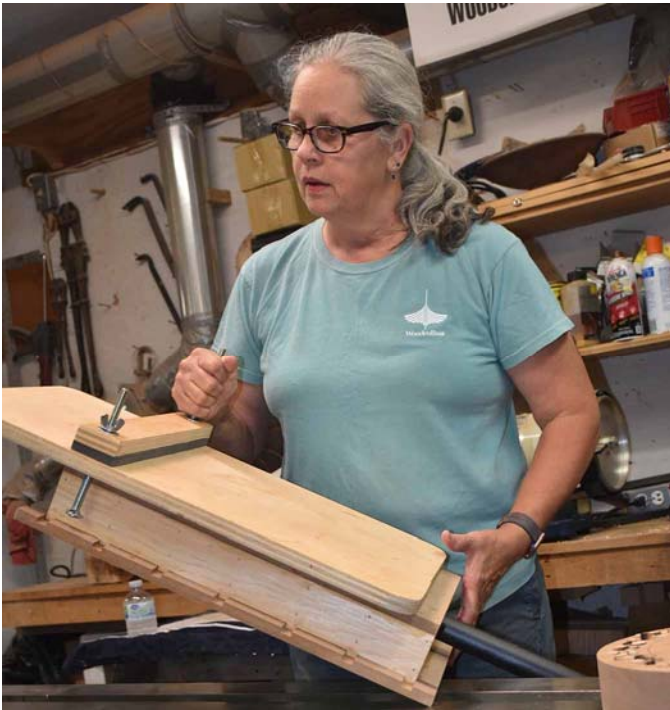
Turn the vacuum cleaner on, block extraneous holes, and your workpiece is tightly clamped.
