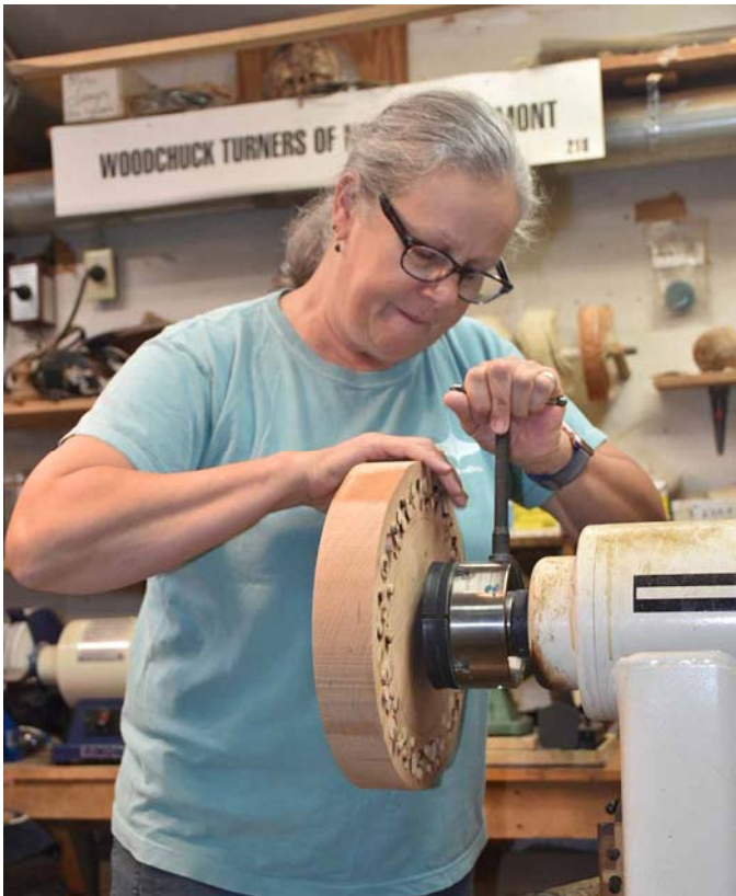
Here, Janet mounts a blank using a screw chuck. Her next step in making one of her signature decorated platters is to true up the edge and start forming the outside & base.
